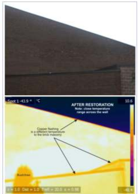
After Restoration (Uniform wall temperature)
