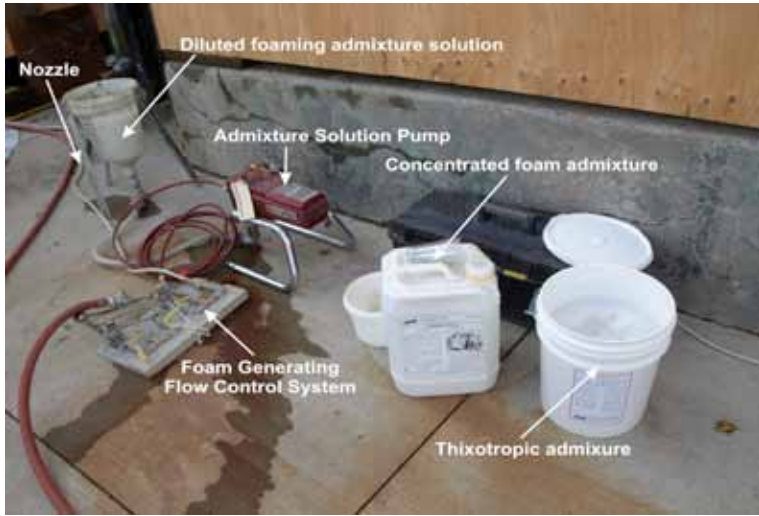
Figures 8 and 9. Left: Equipment and materials for generating foam. Right: Equipment set up for producing foamed grout.
