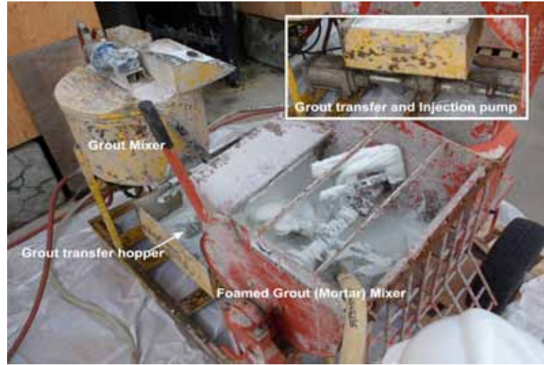
Figures 8 and 9. Left: Equipment and materials for generating foam. Right: Equipment set up for producing foamed grout.
